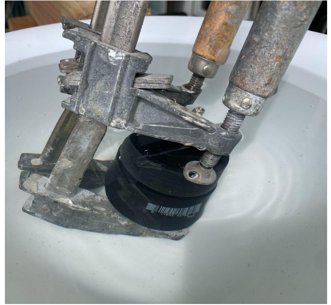
Figure 25: Risk reduction testing rigs for face seal feasibility between the membrane and a face plate
