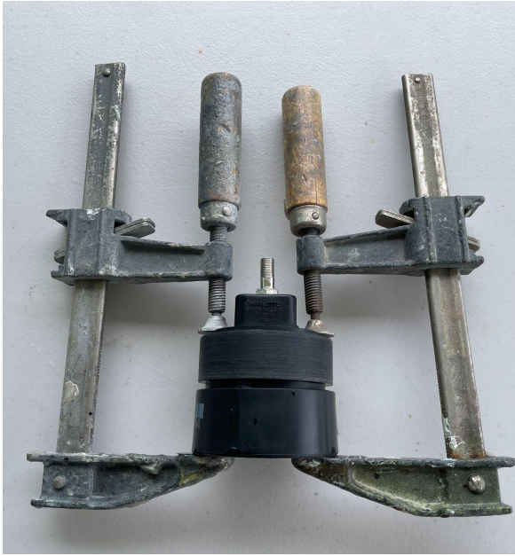
Figure 25: Risk reduction testing rigs for face seal feasibility between the membrane and a face plate
