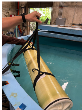
Figure 26: Membrane held in testing tank of saltwater
